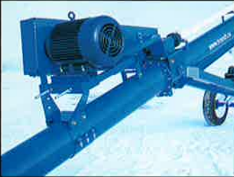
Tube-mount electric belt drive; standard electric belt drive
