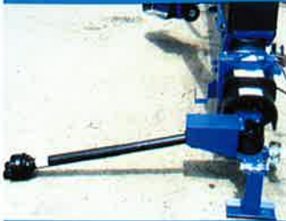
Right angle drive for Swing Away Auger
